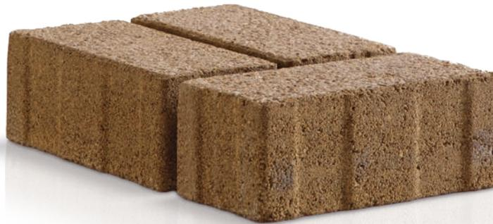
With a striking bush hammered finish, exposing sparkling granite and provides an excellent skid / slip resistance. Specially designed incorporating a slot and chamfer, allowing water to permeate through the finished surface at a high rate. Recommended lay - 45° or 90° herringbone for all trafficked areas. The Ecogranite Aquaflow block can be specified for all sites designed under BS7533-Pt13. Full ancillary kerb system to complement range is also available.
